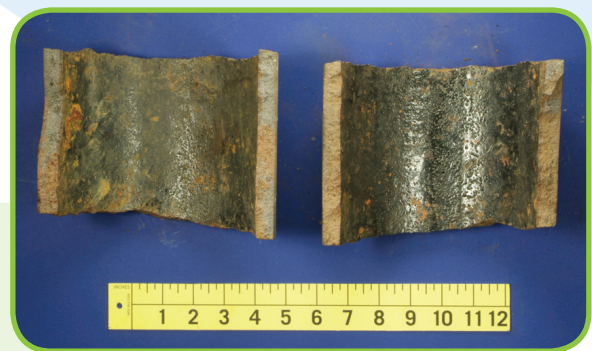
Cross section of extracted pipe sample from site #6
