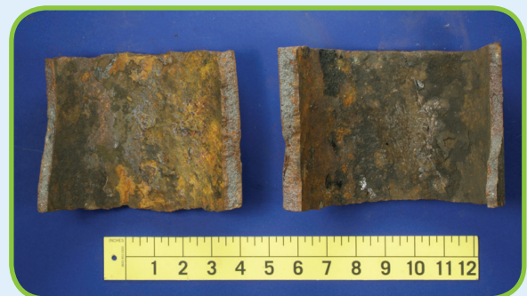
Cross section of extracted pipe sample from site #7
